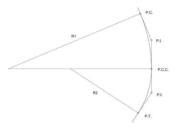
The flatter radius (R1) should not be more that 1.5 times that of the sharper radius (R2).
